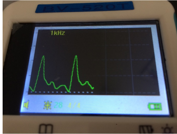
Figure 3 Display of centerline flow velocity profile from the Doppler Ultrasound Scanner
